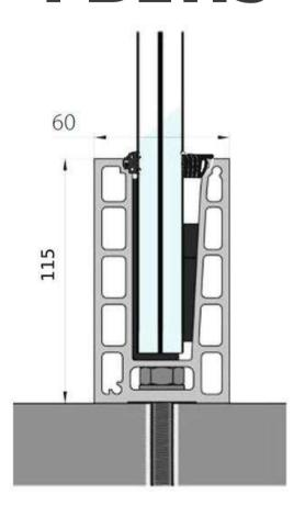
FEATURES: LENGTH: 6000MM HEIGHT: 115MM WIDTH: 60MM WEIGHT: 4.33KG/ML ALUMINUM: EN AW6060 COLOR: STAINLESS STEEL, ANODIZED, RAL COLORS GLASS COMBINATION:
